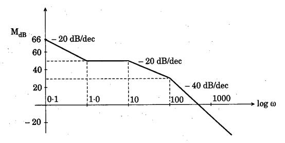
An approximate Bode plot of magnitude for a system was obtained and is shown below. Identify the system in terms of minimum phase transfer function.
