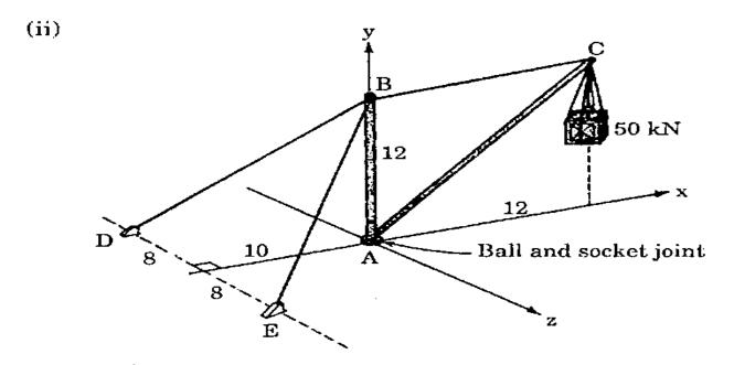
The crane shown in Figure above is supported by cables BD and BE. The distances marked are in m. What are the tensions in the cables BC, BD and BE, when BC is parallel to the x-axis?
