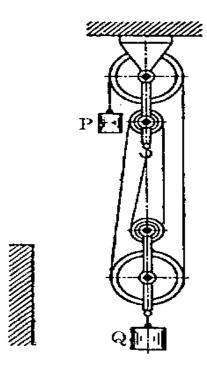
Figure shows a polyspast lifting a weight Q equalling 1000 N by another weight of P equalling 300 N. Neglecting friction and the masses of the pulleys and cables and the inclinations of cables, determine the distance moved by Q in 2 seconds from start.
