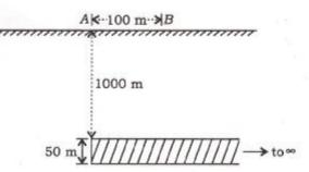
A semi-infinite sheet of thickness 50 m, density contrast 2500 kg/m<sup>3</sup>, lies at a depth of 1000 m. What will be the gravity anomaly at point B which is located at a distance of 100 m from point A as shown in the figure above?
