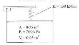
A piston-cylinder device contains 0.05 m<sup>3</sup> of a gas initially at 200 kPa. At this state, a linear spring that has a spring constant of 150 kN/m is touching the piston but exerting no force on it. Now heat is transferred to the gas, causing the piston to rise and to compress the spring until the volume inside the cylinder doubles. If the cross-sectional area of the piston is 0.25 m<sup>2</sup>, determine (i) the final pressure inside the cylinder, (ii) the total work done by the gas.
